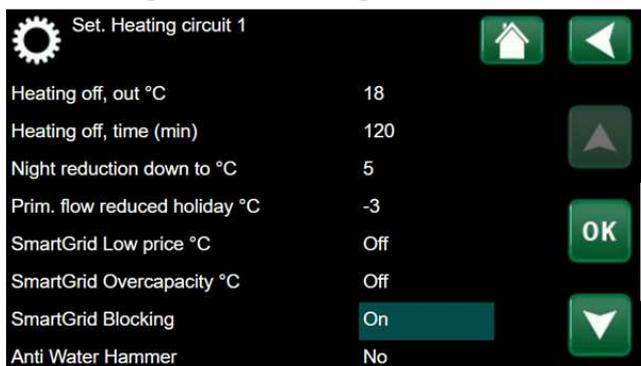
Menu "Installer/Settings/Heating circuit/Heating circuit x"
