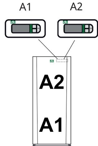
The left-hand display is connected to the bottom cooling module (A1) while the right-hand display is connected to the top cooling module (A2).
