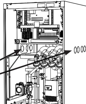
**!** When a collector is connected, the opening must be lined with the edge moulding provided to prevent abrasion of the hose.
