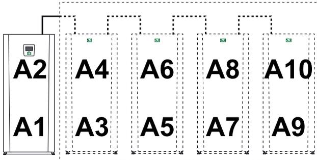
The last heat pump (the cooling module) connected in series must be partly terminated and the shielding in the communication cable must be connected to earth, see below.
