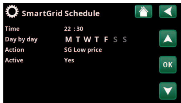
The SmartGrid function "SG Low Price" is scheduled for weekdays 22:30-06:00. Go to the menu by selecting "SmartGrid schedule" in the "Installer/Settings" menu.
